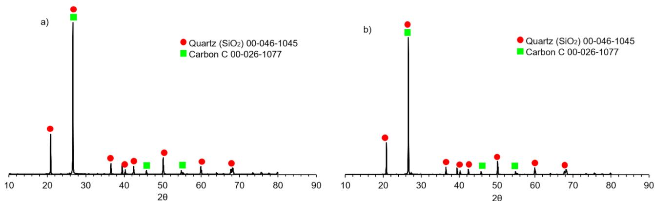
**Figure 2. Diffraction patterns for samples a) 100 and b) +100, after removal of calcium carbonate.**
