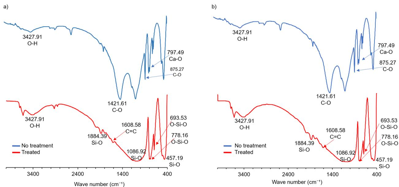
**Figure 3. Infrared spectra of the samples a) 100 and b) +100, before (blue line) and after treatment (red line) to remove calcium carbonate.**
