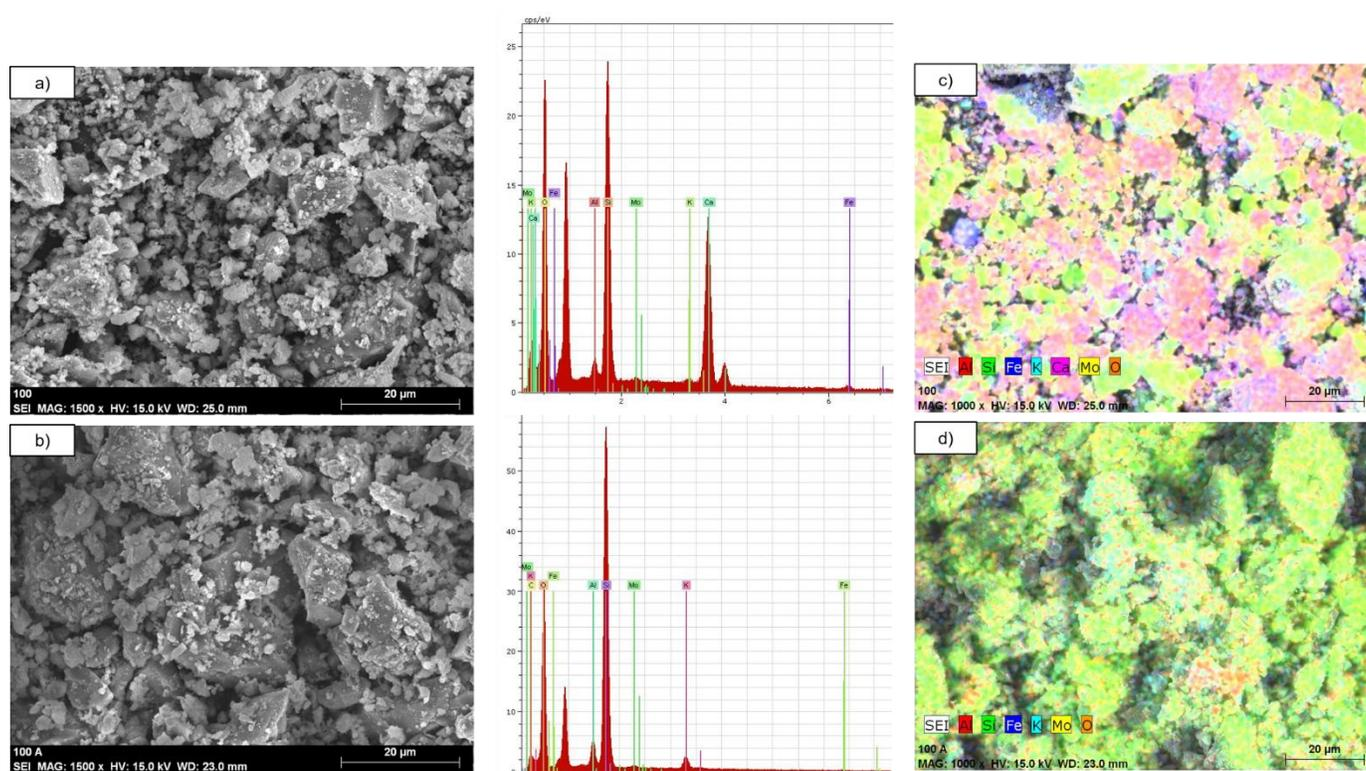
**Figure 4. Analysis of sample 100 by SEM: a) Micrograph and EDS before treatment, b) Micrograph y EDS before treatment, c) mapping before treatment, and d) mapping after treatment.**
