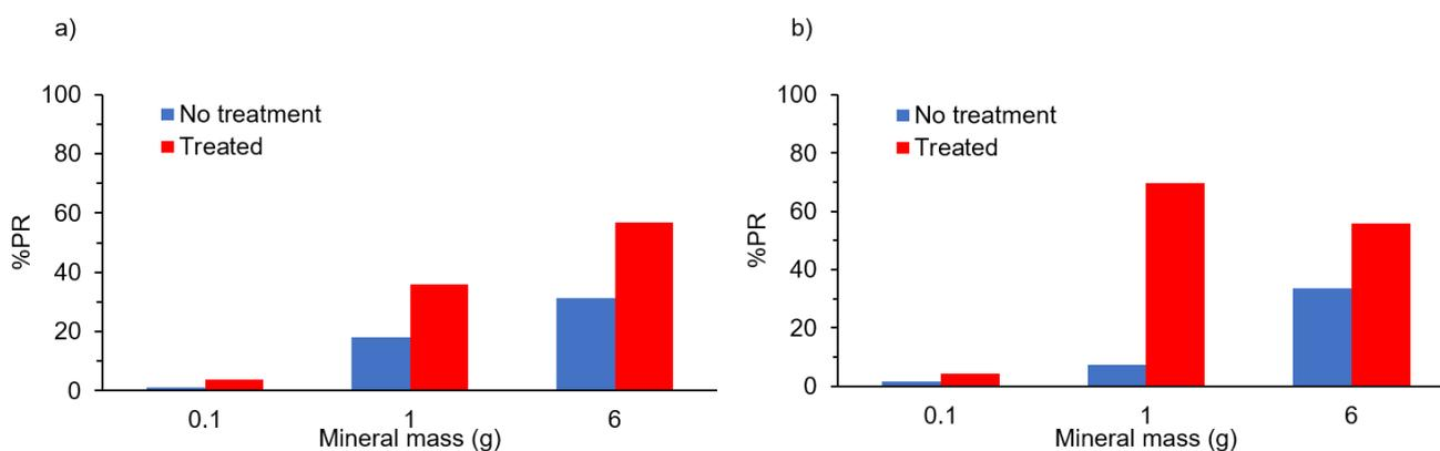
**Figure 6. Preg-robbing degree (% PR) as a function of ore mass for sample: a) 100 and b) +100, before and after inorganic carbon treatment.**
