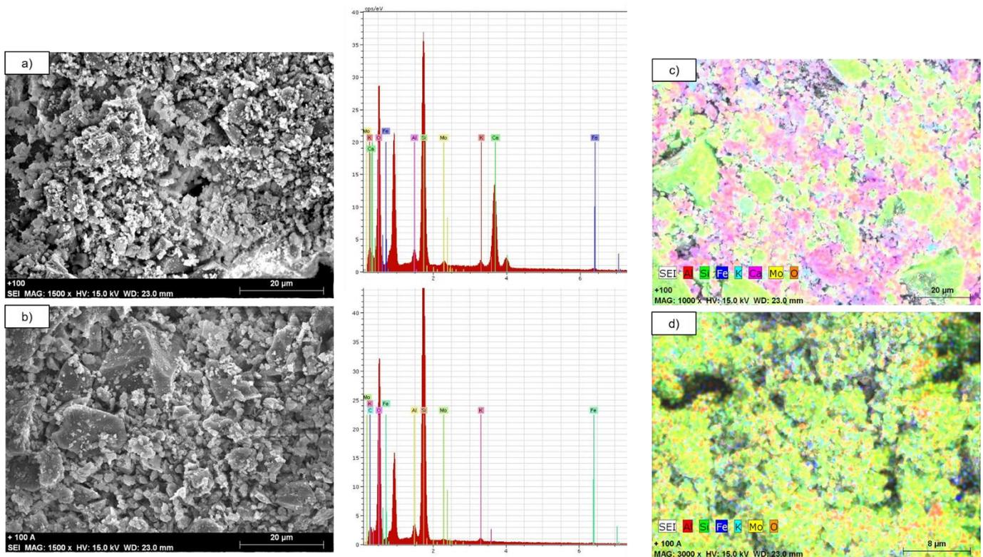
**Figure 5. Analysis of sample +100 by SEM: a) Micrograph and EDS before treatment, b) Micrograph y EDS before treatment, c) mapping before treatment, and d) mapping after treatment.**
