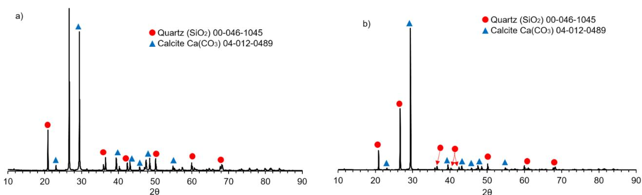
Figure 1. Diffraction patterns for carbonaceous ore. a) 100 and b) +100.
